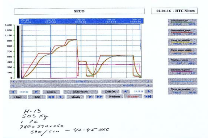
Figure 1. Shows trend graph (units in °C) of hardening with Isothermal quench H13 Die 1100 lbs after two tempering 42-45HRC
