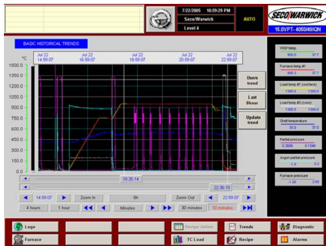
Figure 2. FineCarb low pressure carburizing process cycle
