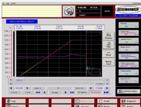
Fig. 2. The process of final sintering in the vacuum furnace type VPT
